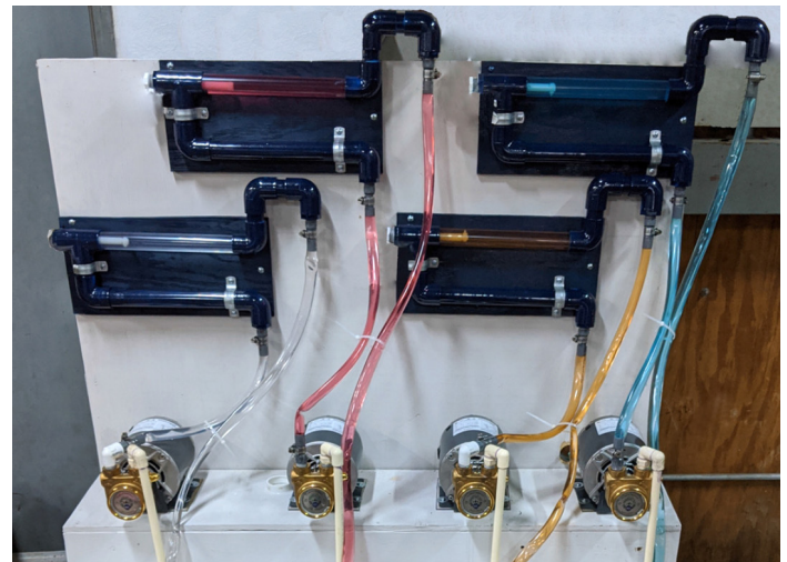
FIGURE 7. Flow-loop system used to simulate a fire suppression system. Antifreeze fluids were inoculated with sulfate-reducing bacteria (SRB), desulfovibrio vulgaris .
